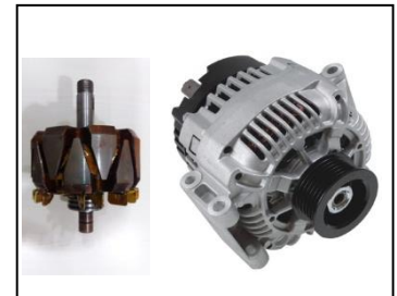
The claw pole rotor made using Fe-P alloy developed at ARCI and the prototype alternator using the rotor
